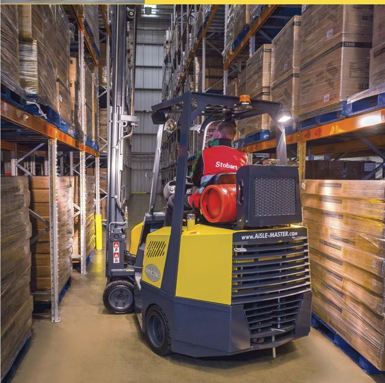
• Hydrostatic drive • Closed loop fuel system as standard
